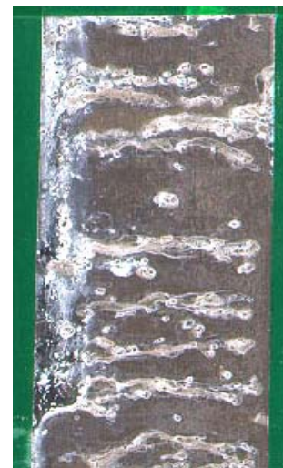
Uncoated 7075 Al After Salt Fog Testing (Fail)
