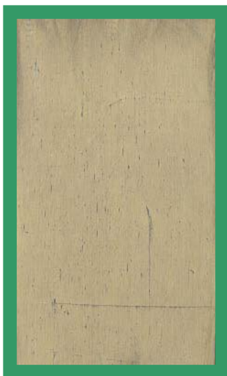
Cerium Oxide Coated Al 7075 Panel Before Salt Fog Testing
