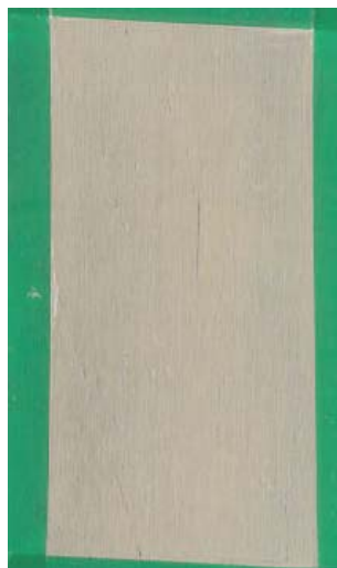
Cerium Oxide Coated Al 7075 Panel After Salt Fog (Pass)
