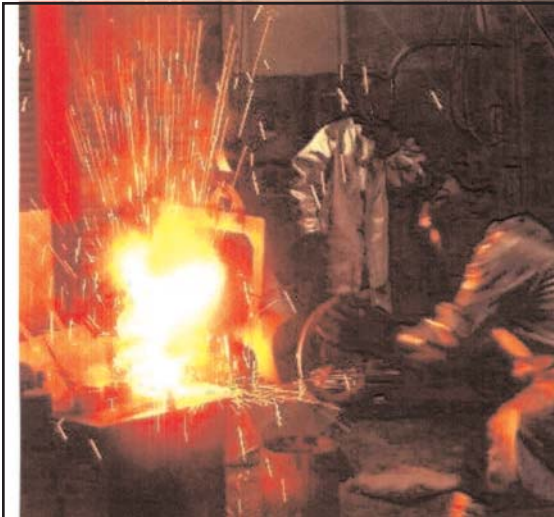
Students Abhay Singh and Jeremy Bryant pour steel in lost foam molds with data acquisition, one of the E-SMARRT programs.
